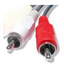
These are also analogue but are not professional. They carry both video and audio signal. It is also a coaxel however, because it has a thin cable it is vulnerable to interference. The RCA does not have the insulated sheath which makes the BNC the better option.
